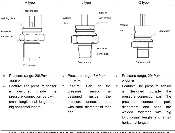
Note: Above are 3 typical structures of all welded pressure sensor. The product is a customized product. Detailed specifications follow customer's requirements.
