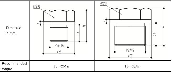
Note: Torque depends on various factors such as material of gasket, supporting materials, lubrication of thread and pressure.
