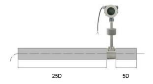
If the upstream of sensor mounting point with two 90 degree elbows is in the different plane, then the length of upstream straight pipe should not be ≤40D, the downstream should not be ≤5D.
